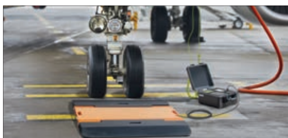
Weighing of airplanes to calculate the loading scheme and determine the centre of gravity, to make sure that the permissible total weight is not exceeded and that the load is correctly distributed
