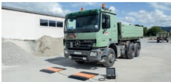
Weighing of trucks, motor homes, trailers etc. for carrying out quick checks of axle weights in any location (Police), to detect and avoid incorrect loading or overloading
