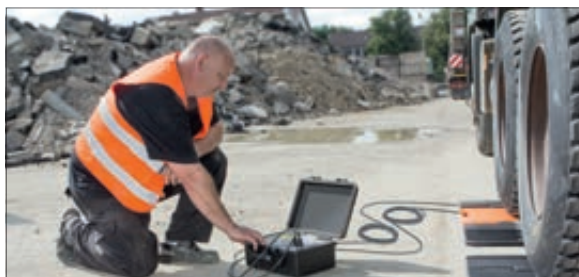
Weighing of tractors, trailers, trucks etc. for products and goods control at the point of receipt or dispatch in locations where there is no permanently installed vehicle scale or one is not available for financial reasons
