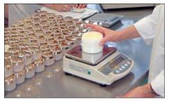
Percentage determination: makes it possible to store a given weight value (100%) and to determine deviations from this target value
