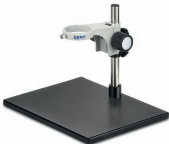
OZB-A5114 with rust protection iron stage
