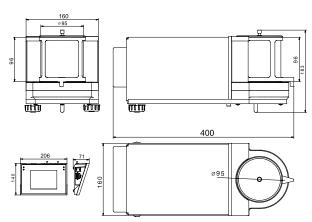
Microbalances MYA 3Y series are intended to measure mass with the highest accuracy. They feature 5,7" LCD colour touch panel which provides new possibilities of balance operation and presenting measurement results. Measurement reliability and accuracy are maintained by system of automatic internal adjustment / calibration.
