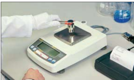
2 only PBS: Adjusting program CAL for quick setting of the balance accuracy, external test weights at an additional price
