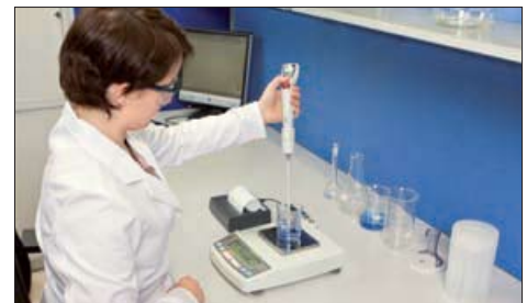
Percentage determination: makes it possible to store a given weight value (100%) and to determine deviations from this target value
