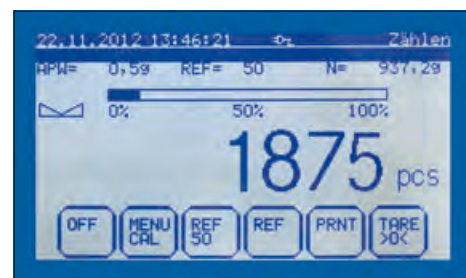
Professional counting function All relevant counting information at a glance, such as, for example, reference weight, reference quantity, total count, total weight, tare container weight, available weighing range and much more Order Hotline: Go to back page of catalogue
